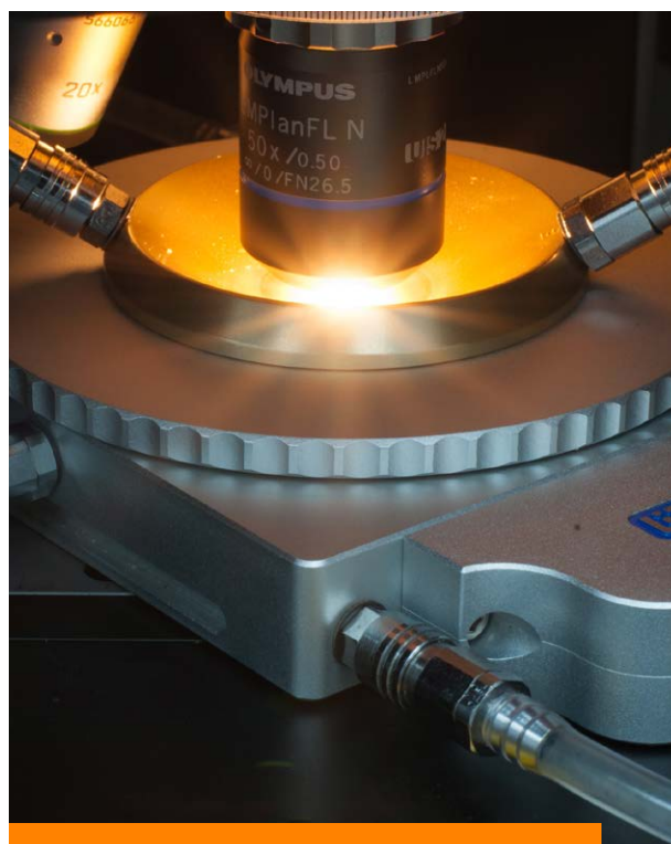
Using LiveTrack focus-tracking to maintain focus on the surface of a sample in a high temperature cell.
