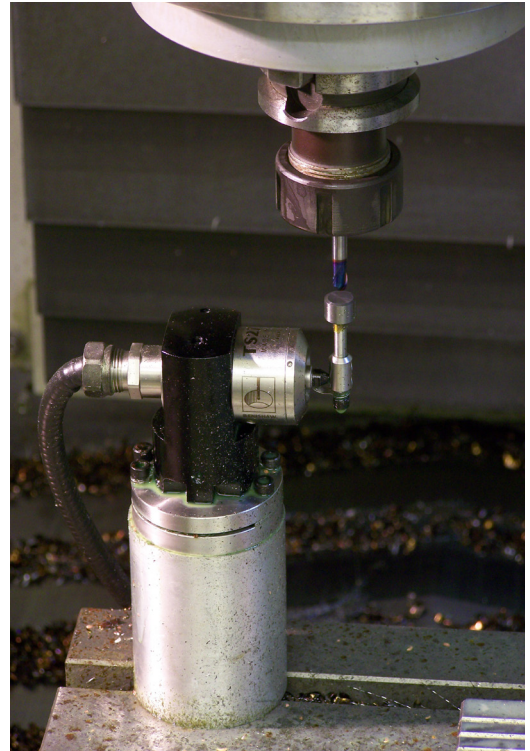
Fast and accurate on-machine tool setting gives consistent results and takes into account thermal effects
