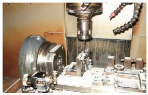
The OMP60 and OTS optical tool setting probe on a machine tool at **Associated Tooling**
