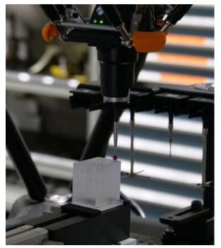
Precision wedge component being scanned on Equator gauging system
